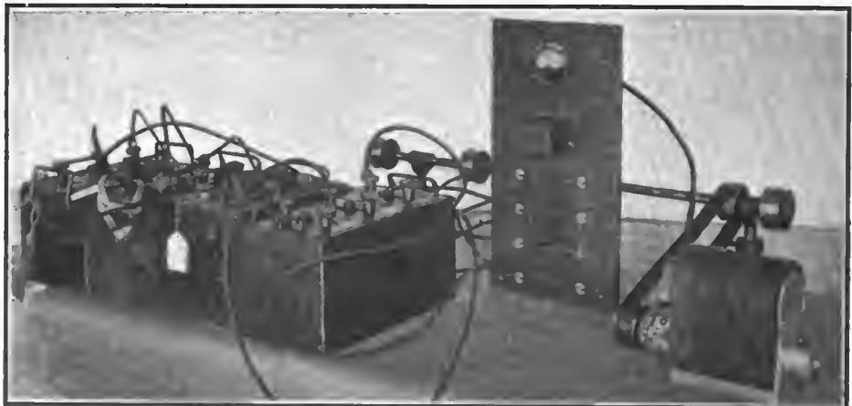
Fig. 7—Esterline charging generator suitable for charging 6 and 12-volt batteries. The generator is driven from a motor by a belt
